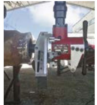
SDB end prepping pressure vessel
