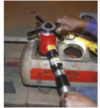
Box header beveling with SDB
