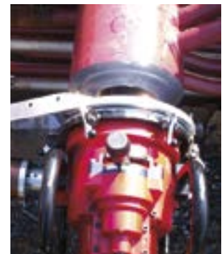
EP 424 SpeedPrep™ deluxe prepping heavy wall pipe
