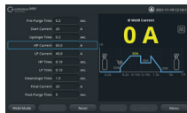
Interface Manual welding
