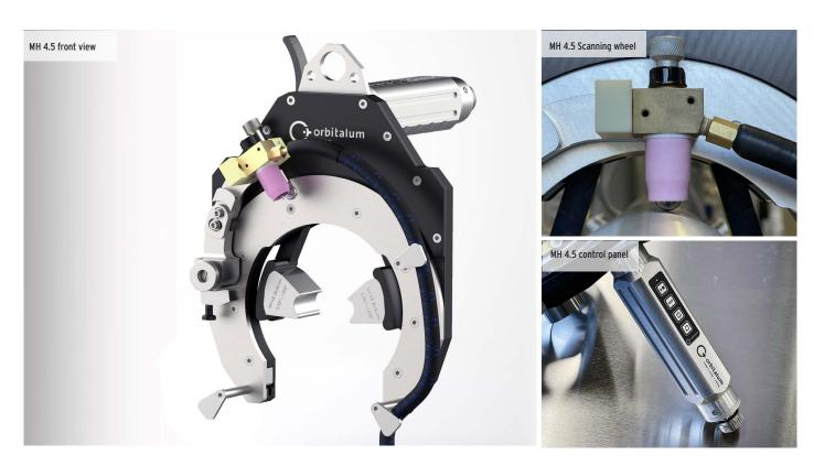
The open orbital weld heads of the MH series are used wherever thin-walled stainless steel tubes are welded in tube installation. They have a compact design and are equipped with a narrow weld head housing with the result that it is possible to weld even under narrow conditions. The Mobile Head is compatible with the orbital welding power supplies of the SW series and the Mobile Welder.
