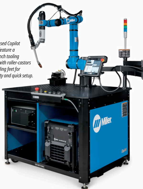
Air-cooled Copilot shown with Auto Deltaweld 350, touch sensing and through-arc seam tracking.
