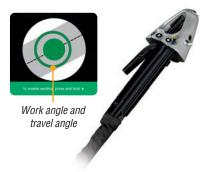
**SmartStinger** extends training capabilities to the SMAW process. LiveArc guides pre-weld positioning for travel and work angles via the LiveArc display.
