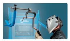
**Welding positioning arm** allows for training in out-of-position GMAW, FCAW and SMAW applications.
